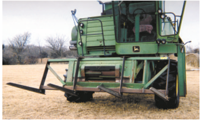
Double forks that replaced header were made with 1/2-in. steel.
