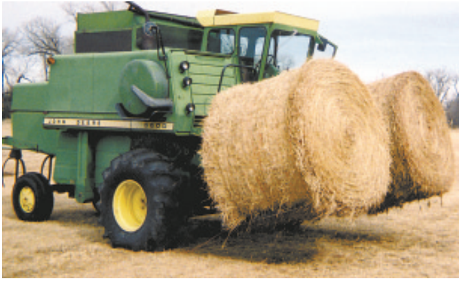
Chuck Misek wanted an easier way to move big round bales. So he converted an old Deere 6600 combine. It can move two bales at a time.
