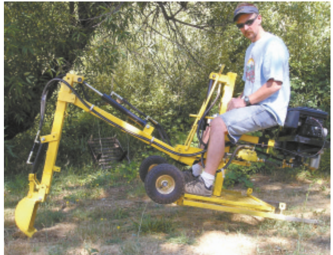
Lonnie Green used his engineering background to design and build backhoes for his own use.
