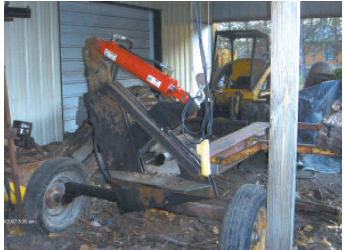
Art Linsenmeyer's powerful hydraulic shear "slices through railroad ties like butter".
