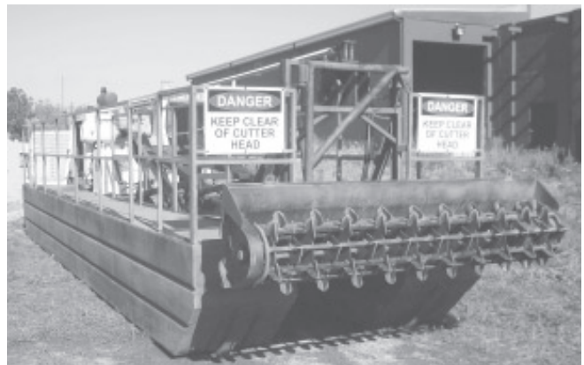
Custom manure applicator Eric Dresbach uses a dredge to get to the bottom of lagoons, pumping up the sludge and sand that often reduces a lagoon's volume.
