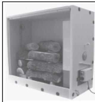
Temporary kilns are made of sheets of 2-in. Styrofoam, held together with clips and screws supplied with the kit. Can be used to dry sawn lumber or firewood.
