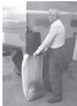
Weaverline mulch bagger is ideal for bagging peat and composted manure. Many customers sell directly from the farm. The bagger holds 2 1/4 cubic yards, enough to bag about 30 2-cubic foot bags.
