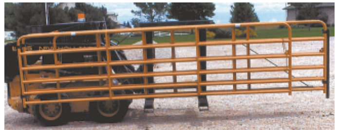
Gate-carrying bracket system lets Tom Hageman use his skid loader to carry up to 50 ft. of connected-together gates at a time, and then quickly unfold the gates for sorting cattle.
