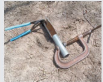
Photos show step-by-step process for converting pipe into trowel.
