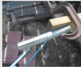
Photos show step-by-step process for converting pipe into trowel.
