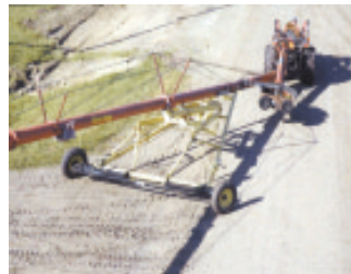
Auger-Steer kit mounts on auger’s axle and is hydraulically-controlled from the tractor. It allows tractor operator to independently steer auger wheels in any direction.
