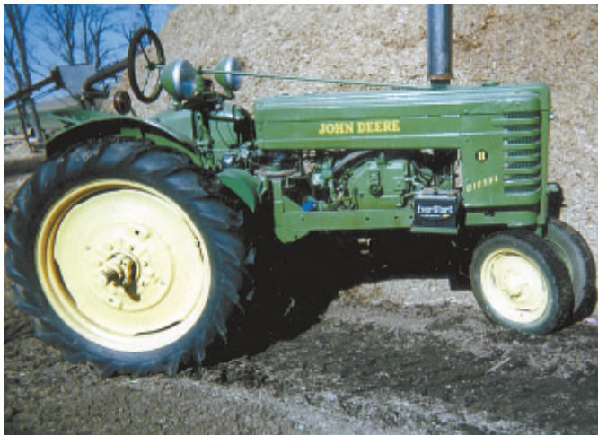
Ben Kinsinger repowered his Deere “H” with a Yanmar single-cylinder diesel.
