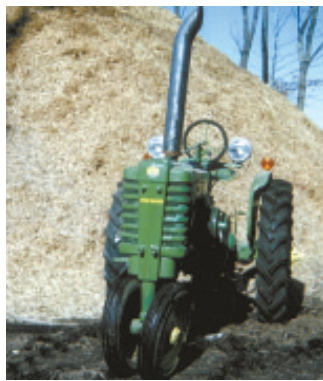
Tractor still has its original exhaust pipe, but it’s hidden from view by a 5-in. dia. chrome pipe off a semi tractor.
