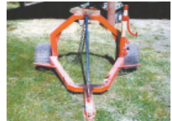
Lift mechanism is a 1 1/4-in. round steel bar with a sliding ring and hook.
