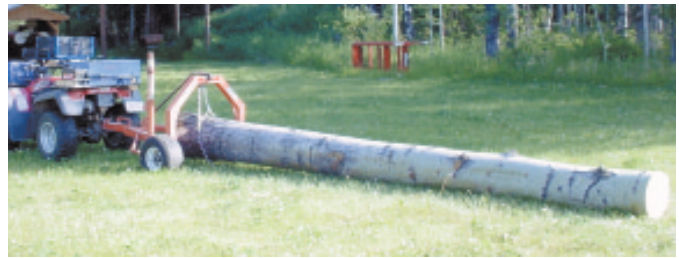
Sidney Stubbs built this heavy-duty log skidder for his ATV. "The biggest log I've hauled was 39 in. in diameter, even though my ATV is only 36 in. high," he says.
