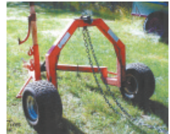
Bar is welded to front of yoke, just behind the hitch and extends back and up at a 45 degree angle.
