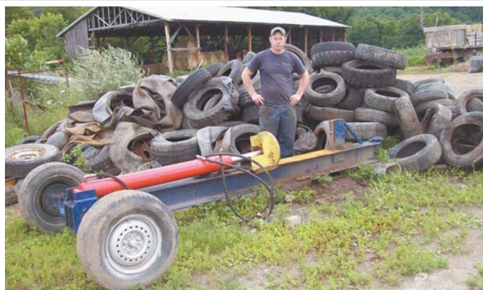
Jeff Overton built this heavy-duty rim crusher out of a giant wood splitter. An "anvil" is welded to one end of rig's 10-ft. long, 10 by 10-in. H-beam.
