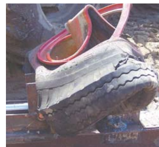
A 5-in. hydraulic cylinder powers a metal plate that crushes tires. Unit is powered off tractor hydraulics.
