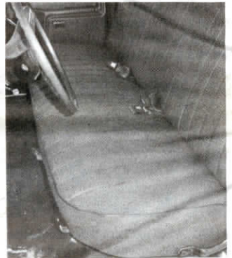
The covering is made of nylon with a 1/2-in. thick foam backing.
