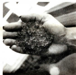
Tiny pile of water-absorbing crystals, upper left, turns into handful of gel, above, when immersed in water-contaminated fuel.
