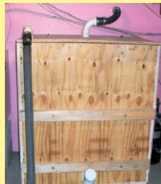
To suck corn into bin, Heinz hooks up a 5 hp shop vac to pvc fitting on bin's lid.
