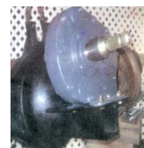
Harry Wallace has figured out a relatively inexpensive way to add 250 to 1,000 hp pto's to semi tractors, using an add-on axle pto.
