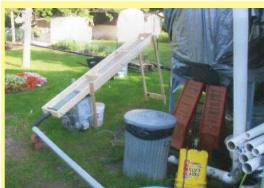
Sifter outside Heinz's house removes fines and a blower gets rid of the chaff. Clean corn flows into a 2-in. pvc pipe that runs through basement wall and into plywood bin inside.
