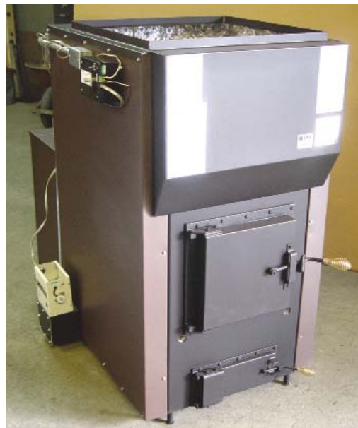
The Kuuma Vapor-Fire 100 hot air furnace recently tested out at 86 percent heat transfer efficiency, 98 percent combustion efficiency, and produced less than a gram per hour of particulates.
