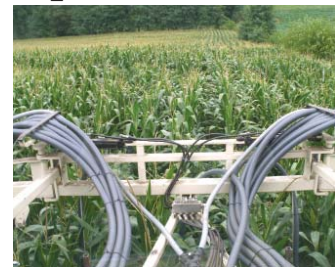
Machine is equipped with an air drill blower and manifold (left) and a 45-ft. boom.
