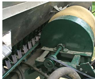
Machine is equipped with an air drill blower and manifold (left) and a 45-ft. boom.
