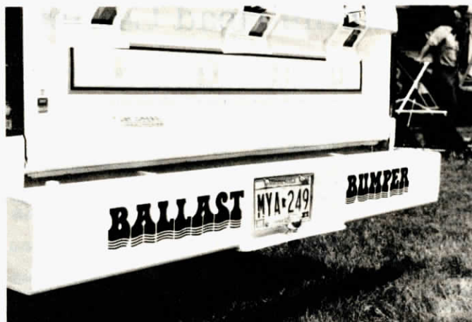
Bumper empty weighs 110 lbs. and holds 110 lbs. of water.
