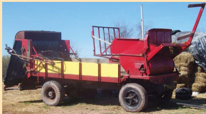
A Vermeer round bale shredder, complete with loading arm, unrolls the bales.
