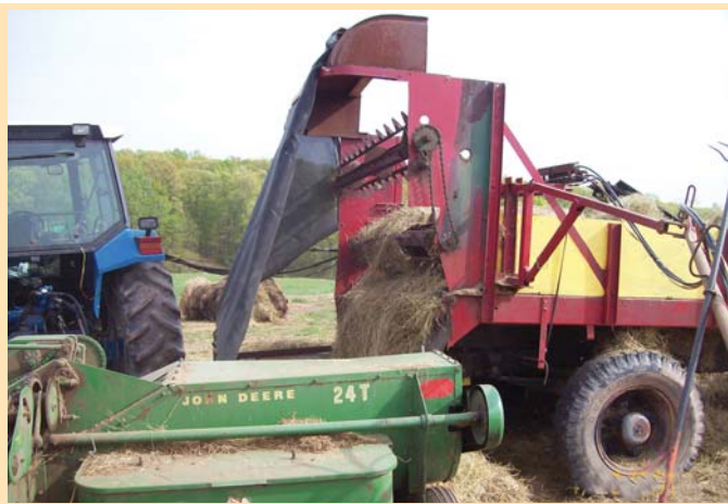
Conveyor floor moves hay to double beaters that fluff the hay, which is then fed into a small square baler. The conveyor and beaters came from a silage wagon.
