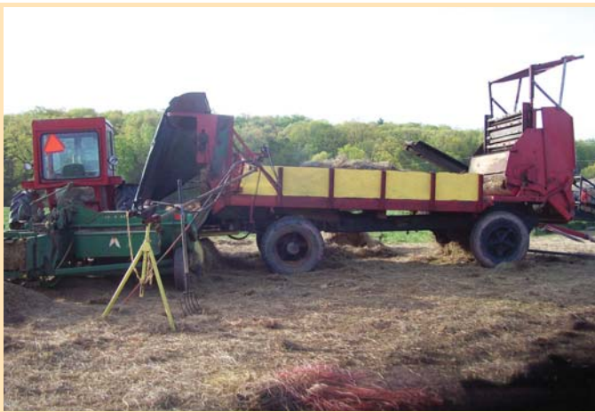
Jay Merriner built this “unroller” that turns big round bales into small square ones. Tripod in foreground is used to control machine’s loading arm, walking floor, and beaters.
