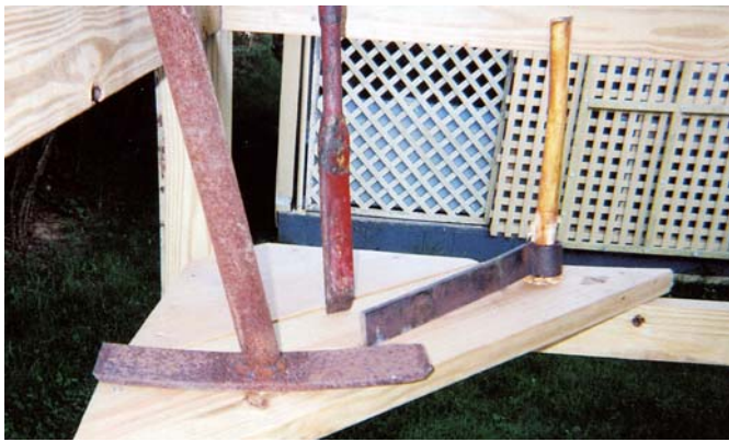
Richard Johnson made some of his car spring tools 50 years ago. Amazingly, he says he's never had to sharpen them.
