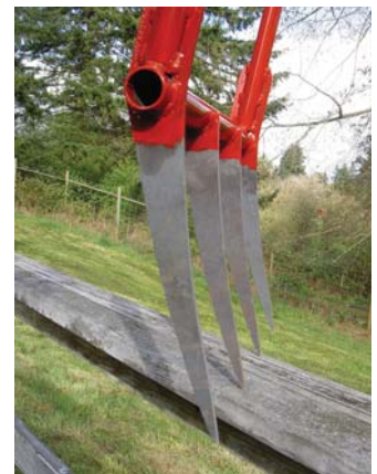
All-steel broadfork eliminates the problem of wooden handles breaking off.
