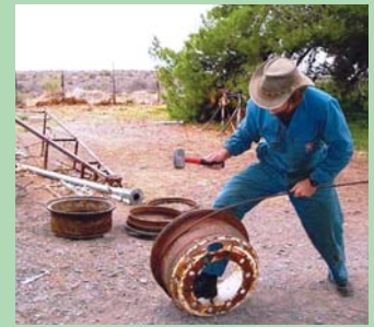
Oakey wraps a steel bar around rim. Stabilizing "feet" (below) are made from scrap pipe.
