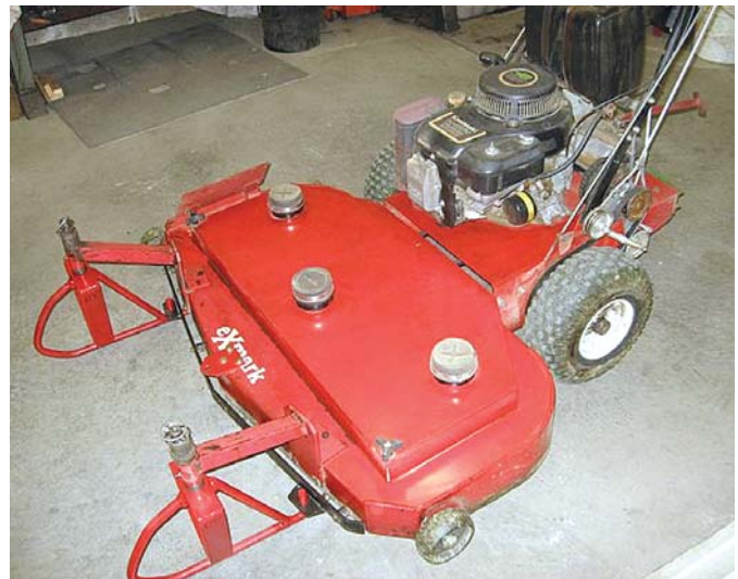
Skids replace walk-behind mower's front-mounted castor wheels, keeping mower from sliding downhill.
