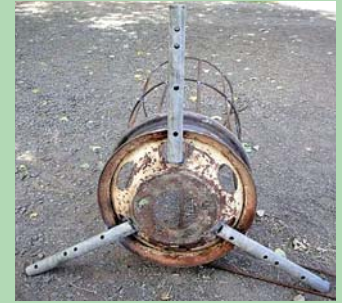
Oakey wraps a steel bar around rim. Stabilizing "feet" (below) are made from scrap pipe.
