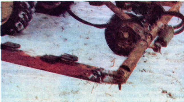
The telescoping hitch arm, and two extra tongues welded to the rake, let you adjust to varying field conditions.
