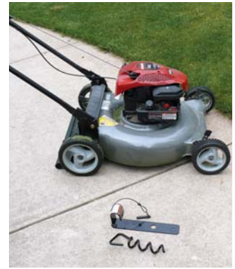
Mower tilt provides safe and easy access to underside of mower without tipping the mower on its side. Mower handle slips under a steel plate (right) secured to lawn with a cork screw stake.
