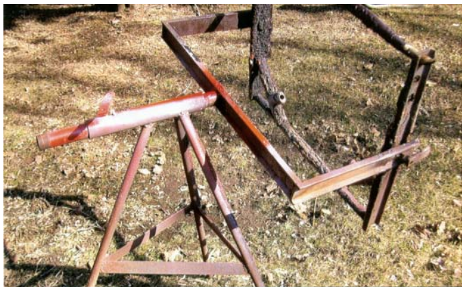
“My wheel holder works great for painting car wheels, because I can turn the wheel in any direction without marking the paint,” says Loren Smith.
