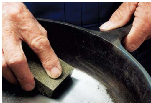
Rubberized abrasive blocks contain silicon carbide grit all the way through, so they never run out of sanding power.
