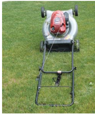
Mower tilt provides safe and easy access to underside of mower without tipping the mower on its side. Mower handle slips under a steel plate (right) secured to lawn with a cork screw stake.
