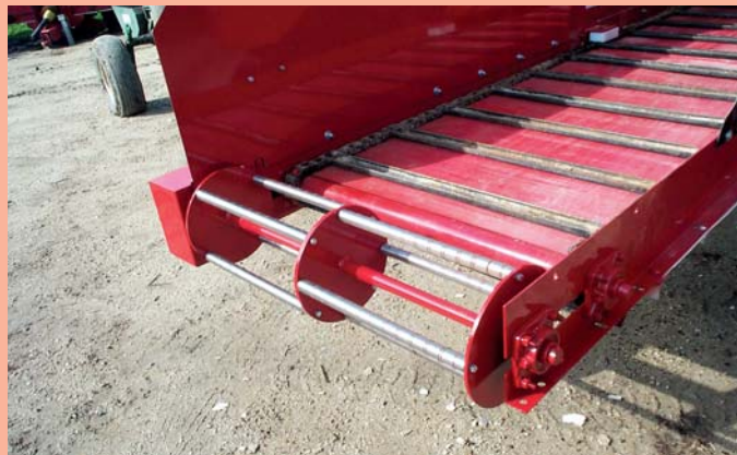
Rotating reel of magnetic bars agitates feed as it flows over, pulling out significantly more metal than standard magnets.
