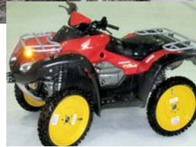
ATV-mounted motocross-style wheels leave a 4 to 5-in. trench up to 12 in. deep that stays open longer. The motorcycle tires make for smooth driving on the road.
