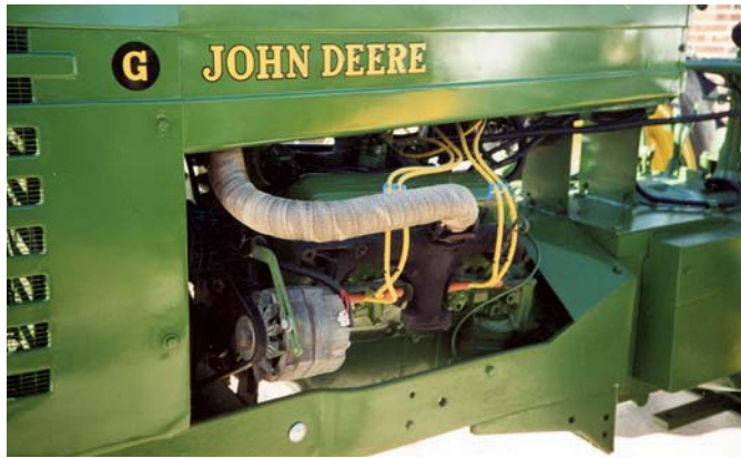
"It took about 2 months to complete the job," says Charles Krieg, who repowered his 1951 Deere "G" with a 327 V-8 out of a Massey 510 combine.
