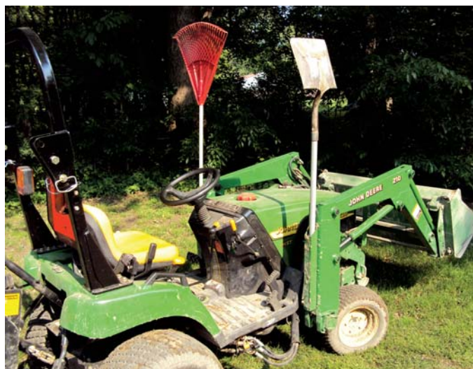
Joe Campoli used 2-in. sq. tubing to make shovel and rake holders for his utility tractor.
