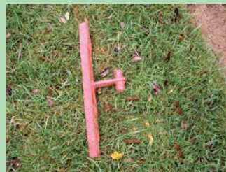
Anti-lift bar keeps 3-pt. drawbar from accidentally lifting when towing a cart.
