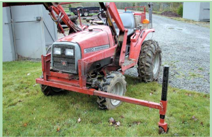
Adjustable height caster wheel mounts on a steel leg, which slides through a sleeve that attaches to tractor's front end.
