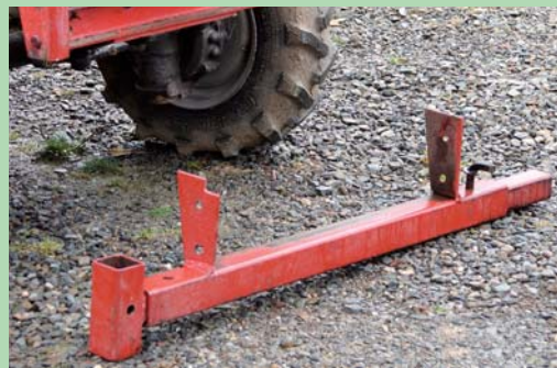
Sleeve is mounted perpendicular to one end of a 44-in. long metal tube. Tabs welded to sleeve bolt onto front-end loader supports.
