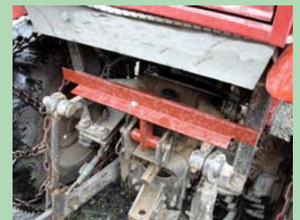
Anti-lift bar keeps 3-pt. drawbar from accidentally lifting when towing a cart.
