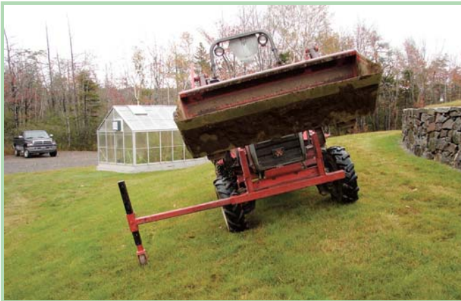
Add-on outrigger slips onto either side of tractor for work on steep sidehills.
