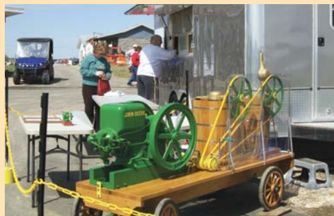
Dan Lang makes sweet corn ice cream, using a 3 hp Deere hit and miss engine that drives two 5-gal. ice cream makers.
