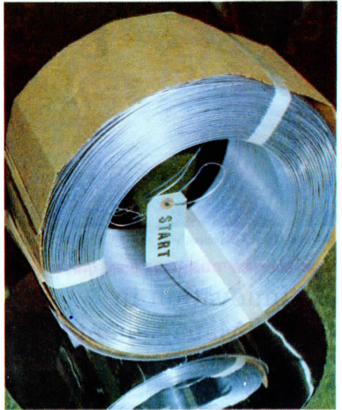
Rolls of 14½ ga. galvanized wire come with both ends of the wire in the center, but only the starting end is tagged. Just punch out the center, grab the tag and pull. You automatically have the starting end.
