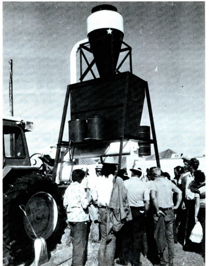
New cuber lets you store hay, roughage in 1/10th less space. Molasses, grain or supplement can be blended into cubes to upgrade feeding value of low-grade roughages.
