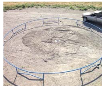
Water drains out of trampoline and is piped into a 7,000-gal. storage tank (left). Tarp stretches across a round metal frame. Note metal drain in ground (right).
