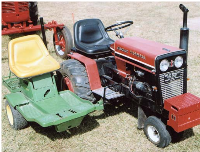
Deere “sidecar” was made by mounting the back half of a Deere riding mower onto one side of a Cub Cadet garden tractor.
