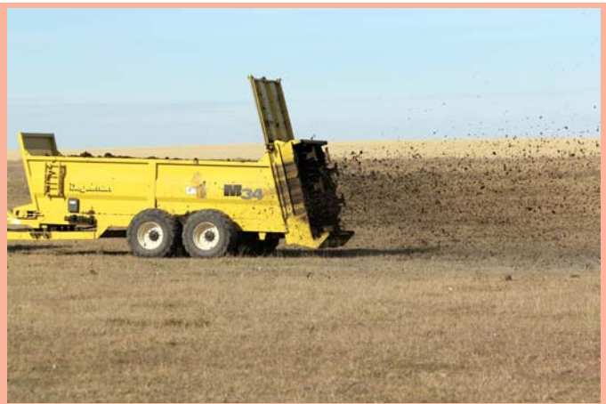
In addition to being big, the spreader has an innovative beater design that eliminates rock damage.
