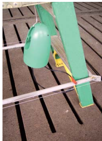
A pair of thin metal cables are spaced 3/4 in. apart and attached to a 1/2-in. dia. pvc pipe, which goes all the way around ladder.
