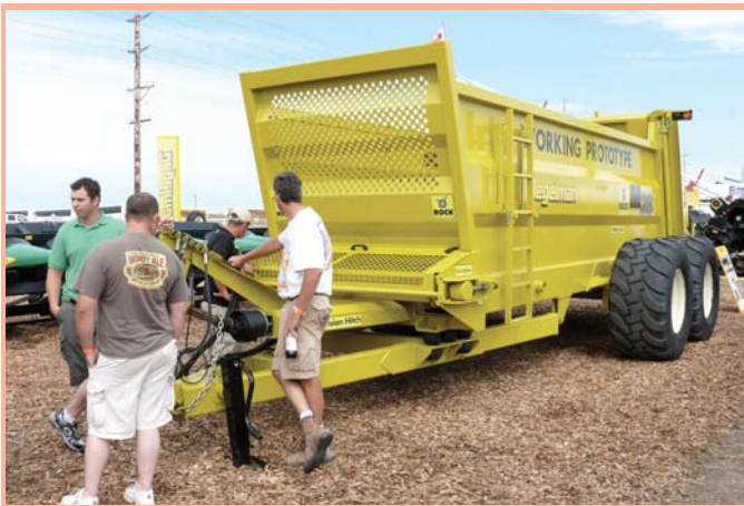
Degelman Industries' new spreader has a capacity of 28 tons. It's designed to move not only manure but also dirt or other material.
