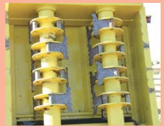
Free-swinging flails have replaceable paddles mounted on 10-in. dia. tubes. Flails collapse if they hit a rock, allowing rocks to pass through without damage.
