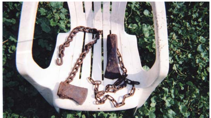
Welded-on safety chain keeps wedge from flying up after being hit.
