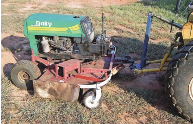
Glenn Fisher pulls his 4-wheeled, self-powered "trail-a-mower" behind his IH Cub 15 hp garden tractor.
