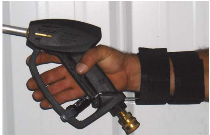
Spring-loaded pressure washer arm brace holds pressure washer's gun trigger in a locked-on position.
