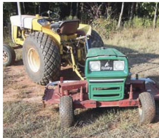
A 60-in. Woods mower deck bolts to underside of tractor, which faces backward.
