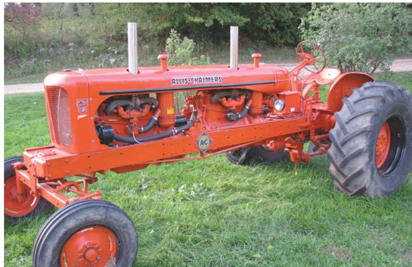
Denis Post’s Allis Chalmers WD 45 tractor is 14 ft. 7 in. long and has two hoods to cover its twin engines. He built the second engine using parts from a half dozen old Allis Chalmers tractors.
