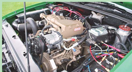
Power is provided by a 4-cyl. Cummins industrial engine with 116 hp. Cab is equipped with a state-of-the-art GPS system (right).
