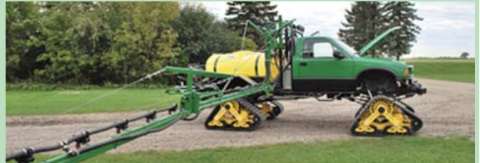
Sprayer features all-wheel-steering, 4-wheel hydraulic drive, a self-leveling air ride suspension system, and front and rear locking axles.
