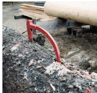
Thibault bark peeler is designed to slit the wood and peel it back, separating the bark from the log (left). Hook is filed down so it’s flat underneath.
