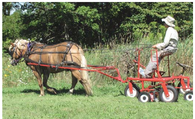
Mini Gang reel mower lets you put a mini horse or donkey to work mowing the lawn.
