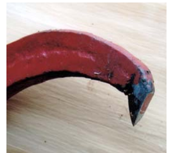
Thibault bark peeler is designed to slit the wood and peel it back, separating the bark from the log (left). Hook is filed down so it’s flat underneath.
