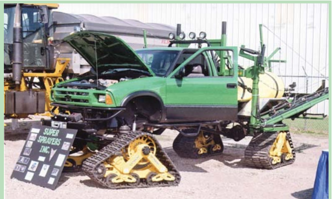
Custom operator Matt Hanson built this 4-WD “super sprayer” to ride on either tires or steel tracks. “It’ll go anywhere, regardless of field conditions,” he says.
