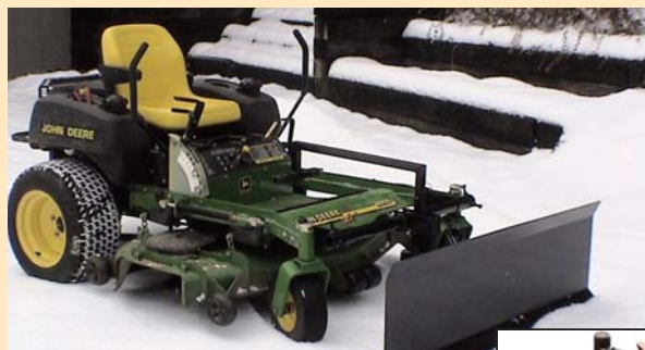
You can turn your zero-turn mower into a snowplow by adding a Universal Mounting Bar, says Country ZTR, other attachments mount on bottom.
