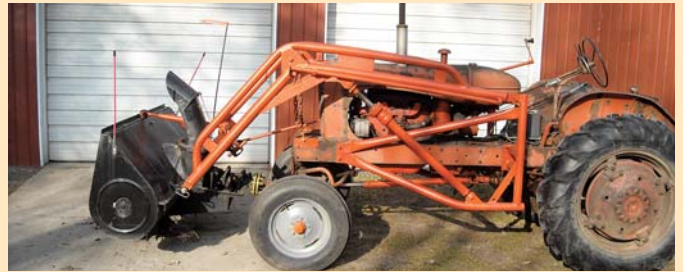
Rick Bezemek rigged up a front-end pto drive on his WD Allis Chalmers tractor and also mounted a used snowblower on tractor's trip-style loader.
