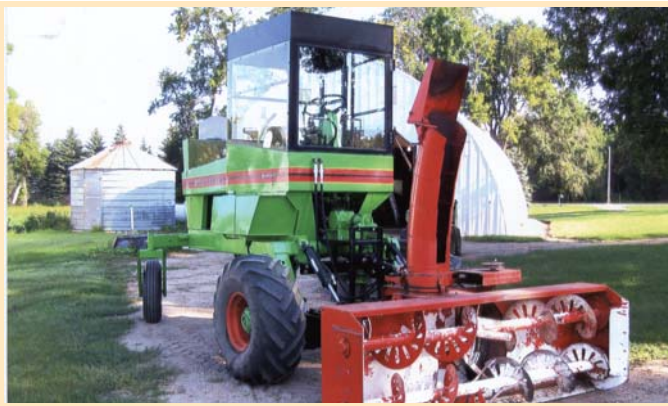
Jeryl Van Der Pol turned an Owatonna hydrostatic-drive swather into a big self-propelled snowblower with a 7-ft. double auger.
