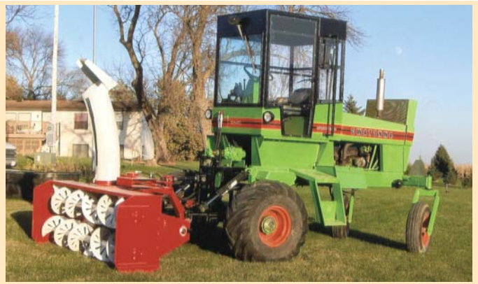
He made his own cab, using safety glass for the windshield and plexiglass for the side and back windows.
