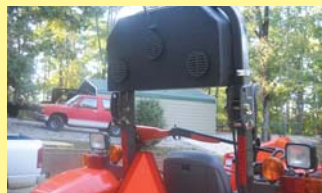
Stereo system components mount on a removable, vinyl-covered "box" that's U-bolted to tractor's rollbar. PVC drain grates on back hold speakers in place.
