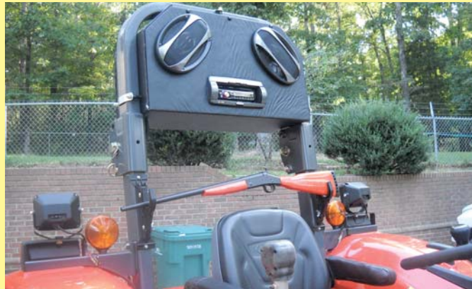
Stereo system components mount on a removable, vinyl-covered "box" that's U-bolted to tractor's rollbar. PVC drain grates on back hold speakers in place.
