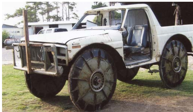
Big wheels increase rig's clearance from 10 to 24 in., which keeps truck from getting hung up in deep mud.
