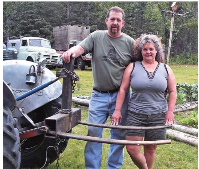
Trent Sexton and his wife Christine use this 3-pt. mounted forklift mainly to haul firewood. It uses a pair of springs off a Kenworth semi tractor.
