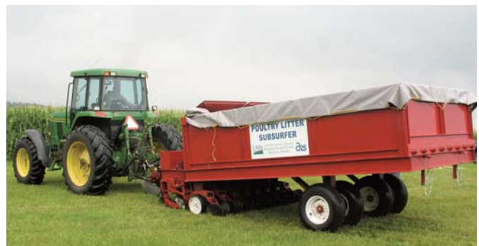
USDA researchers have come up with a machine that grinds up chicken litter and injects it underground. Reduces losses due to volatilization of nitrogen.
