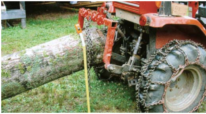
Ralph Thibault built two yokes to fit the 3-pt. hitch on his 20 hp tractor. Yokes keep logs up off ground as he skids them out of woods.
