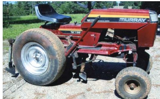
Riding mower is fitted with two cultivator shovels in front of rear wheels and two more behind. Shovels attach to mower deck's original lift linkage.
