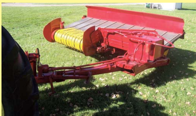
"It fluffs the windrow and can reach deep down into ditches," says Aaron Melby, who built the inverter out of a New Holland 9-ft. haybine.
