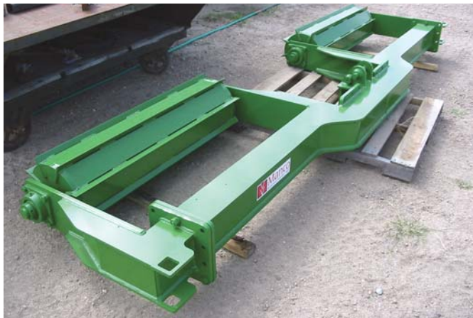
Blades on drums are designed to crush the stalks ahead of tractor tires.
