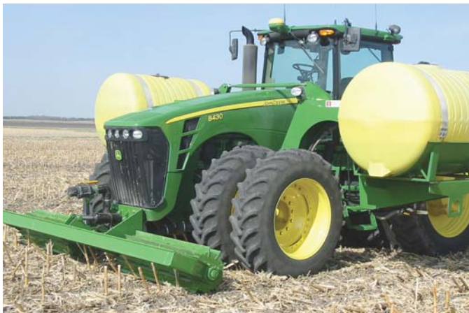
Manco Stalk Roller uses two 500-lb. drums to smash corn stubble. It bolts on in place of weight brackets on tractor's front end.
