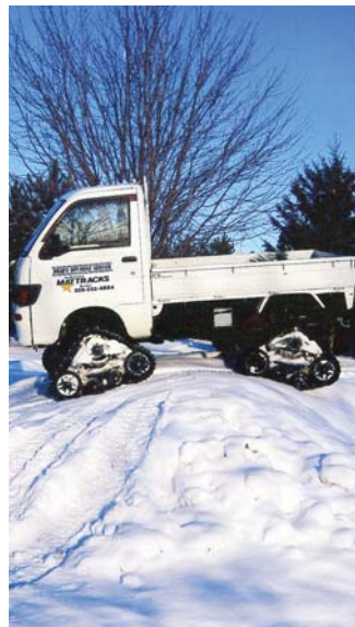
Brad Paul installs Mattracks on everything from ATV's to pickups. Photo shows his own Daihatsu mini truck fitted with tracks.
