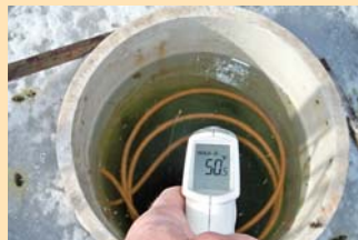
Heat gun shows that water temperature inside pvc drinking tube is at 50 degrees while the rest of the tank is covered with ice.
