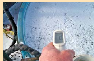
Heat gun shows that water temperature inside pvc drinking tube is at 50 degrees while the rest of the tank is covered with ice.
