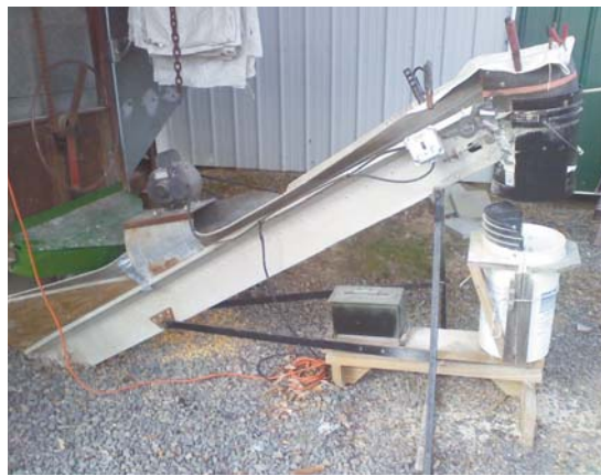
Elevator carries corn to a cut-out 5-gal. bucket, which directs grain into a bag. Bottom of bag lays in a second bucket fixed to a treadle scale board. When bag reaches 50 lbs., board tips and activates a shut-off switch on elevator.
