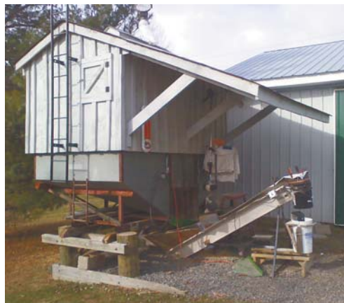
Howard Arnold uses a homemade bagger system with treadle scale to fill 50-lb. bags with shelled corn. System uses a covered gravity box that's filled by an auger.
