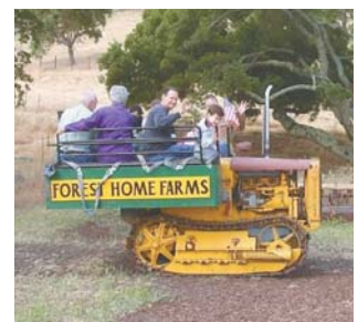
Roy Ginochio built this 10-passenger carrier that mounts on back of an old Cat. Carrier consists of a 7-ft. long box with two side benches and a driver's seat. seatbelts still in the box.
