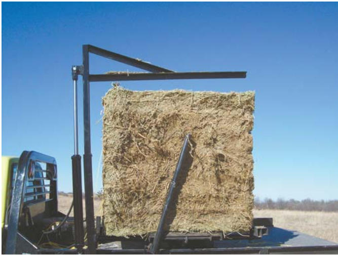
Introduced 12 years ago, the Bale Buddy now comes with a new “flaker” that cleaves flakes off one side of truck and onto the ground.
