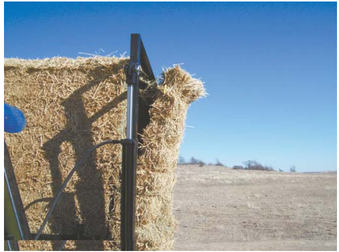
Flaker lets operator precisely control how much of the bale to feed at one time.
