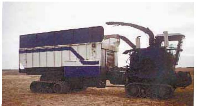
Morgan used components off an existing Deere self-propelled forage harvester, building the chassis from scratch with an articulated steering joint at center.
