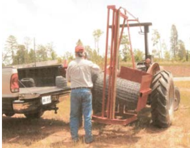
Loading the roll of wire is easy, thanks to a cantilevered loading mechanism on unit.
