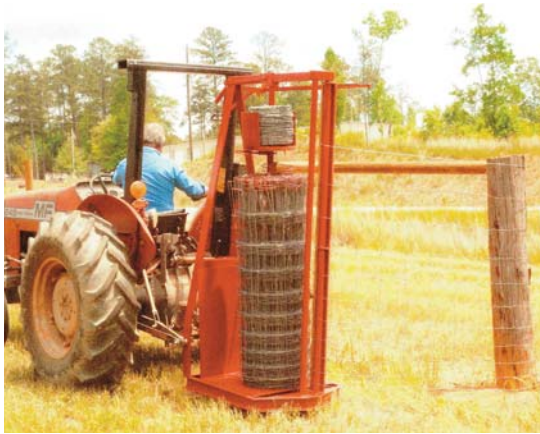
The 3-pt. mounted Fence-Mate holds, unrolls and stretches wire as it goes.
