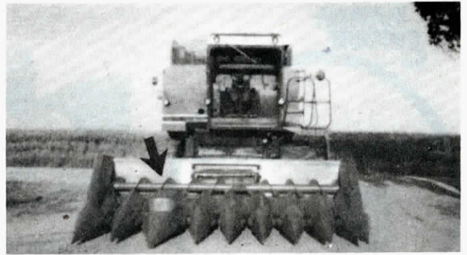
Arrow points to "skip row" snout on this 8-row header for narrow rows custom-built by Harv's Supply.
