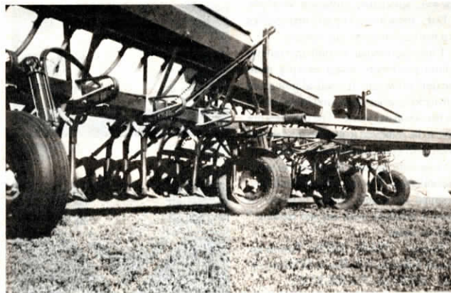
Note the high clearance of rebuilt drills and the 1 1/4-in. drop pipes welded to bottom of "C" shanks.
