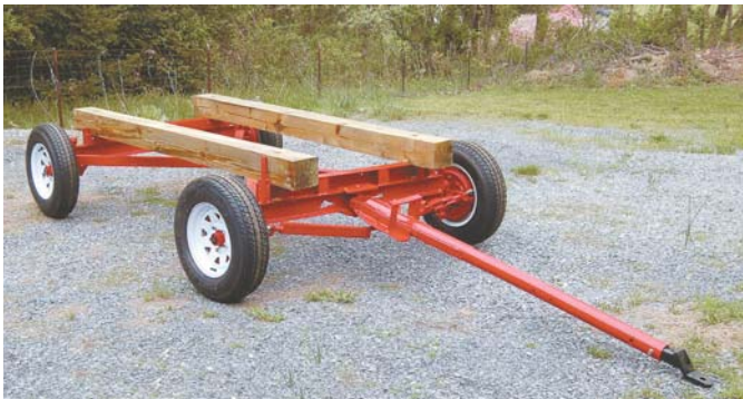
Doug Creswell built a 6 by 10-ft. hay wagon on an old running gear. A pair of 6-in. sq., 8-ft. long wooden beams support wagon bed.
