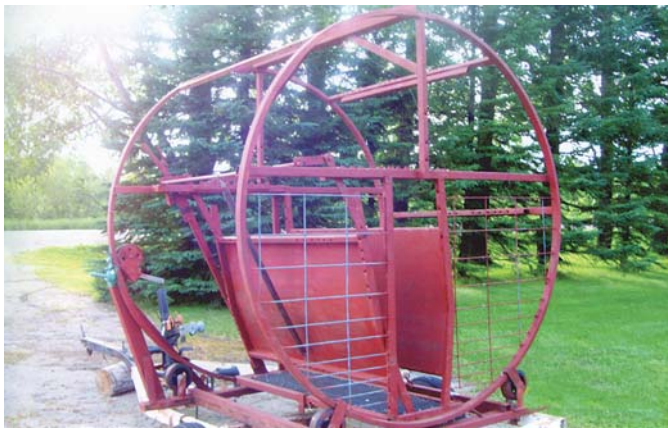
Rolling squeeze chute is made from a wire spool, with a trimming chute at the center. A winch is used to rotate the chute.
