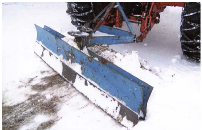
Add-on grader blade is welded onto back of original blade. "It eliminates the need to get off the tractor to rotate the blade," says Sherman Campbell.
