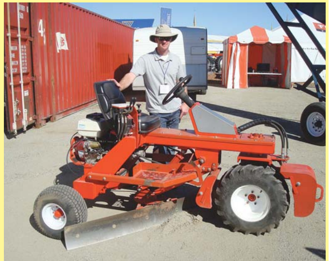
Marcus Benedict's 3-wheel hydrostatic drive grader turns in a 180 degree arc. The single front drive wheel is driven by a hydraulic motor that's powered by a Honda engine.
