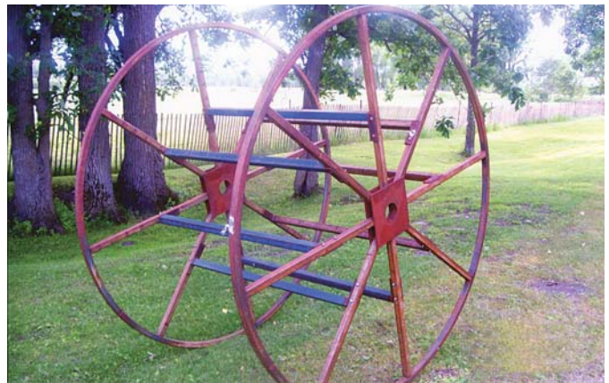
Inventor Roger Holcomb used an empty spool from a local telephone company to build the rolling squeeze chute.
