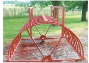
Holcomb also uses cable spool to make big bale feeders for calves, sheep and goats. Photo shows a new feeder upside down for painting.
