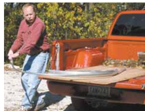
FARM SHOW tested Robinson's simple method of bending hoops to make 4-ft. garden row covers. Bender bolts onto any horizontal or vertical surface that allows room for pipe to be bent from a straight position.
