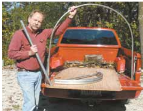
FARM SHOW tested Robinson's simple method of bending hoops to make 4-ft. garden row covers. Bender bolts onto any horizontal or vertical surface that allows room for pipe to be bent from a straight position.
