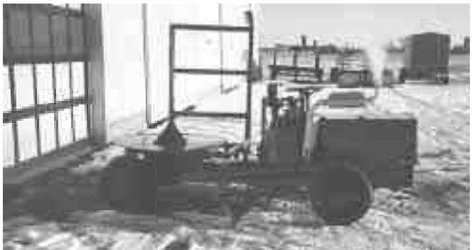
Turntable is powered by a hydraulic motor that's driven by a hydraulic pump belt-driven off the engine. With two in-line mufflers the unit runs quiet.
