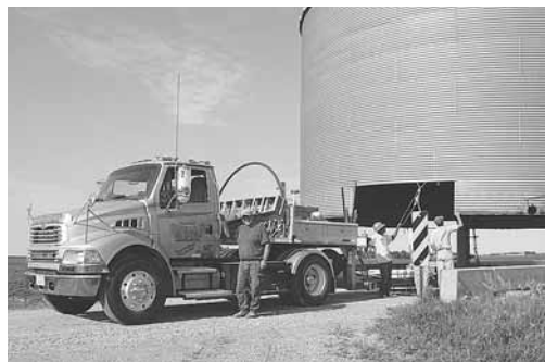
Bruellman and crew pull a 36-ft. dia., 31-ft. high bin over a bridge (left). Top dryer bins are movable, too (below).
