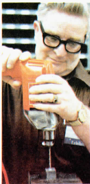
Al Witte demonstrates left hand drill bit.
