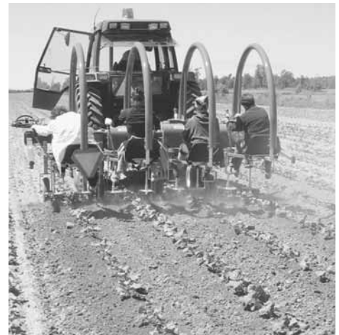
Pto-driven weeder wheels are equipped with rubber-mounted steel rake teeth, which uproot weeds without damaging the crop. A Multiple Row Weeder for 3 to 6 rows is also available (right).
