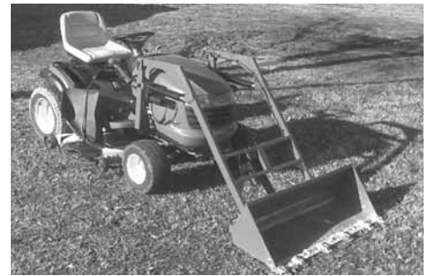
Kelly Loader bucket can be raised up to 48 in. high - enough to load a pickup bed - and dumped. It's operated by three electric linear actuators that hook up directly to the tractor's battery.
