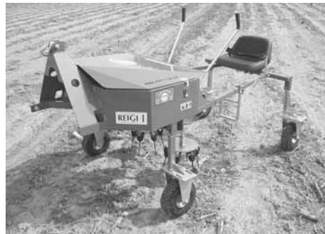
Pto-driven weeder wheels are equipped with rubber-mounted steel rake teeth, which uproot weeds without damaging the crop. A Multiple Row Weeder for 3 to 6 rows is also available (right).
