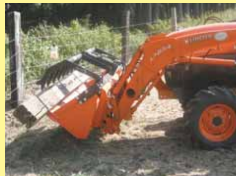
Patent pending ANBO Bucket Grapple, above and below, is fitted with tines that rake in forward or reverse.
