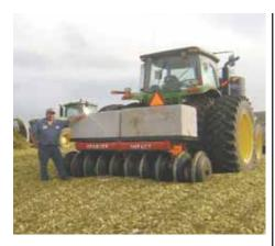
Silage Roller's narrow wheels are custom made for each customer's operation.
