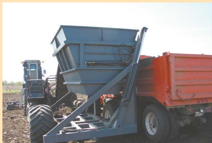
Rocks roll toward the center where they're gathered onto a conveyor and then deposited in a trailing side-dump cart.
