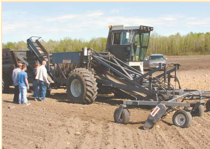
Mel Aho's home-built, self-propelled rock picker uses a New Idea 803C power unit and comes with gathering arms, conveyors and a hydraulic side-dump cart.
