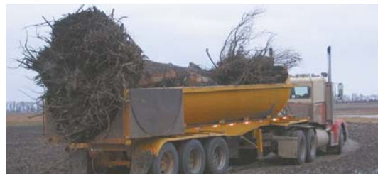
Lyle Carpenter and his son Leeroy built this huge dump trailer out of an old over-the-road propane semi tanker. They use it to haul rocks, stumps, scrap metal and more.
