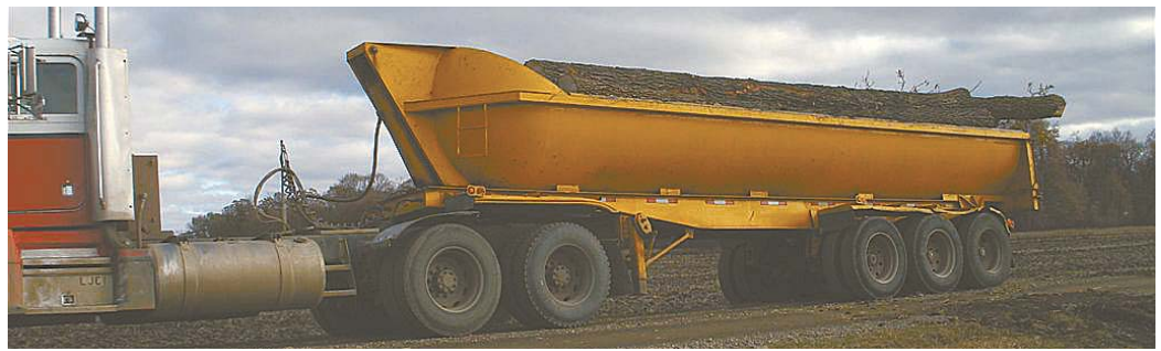
Lyle Carpenter and his son Leeroy built this huge dump trailer out of an old over-the-road propane semi tanker. They use it to haul rocks, stumps, scrap metal and more.
