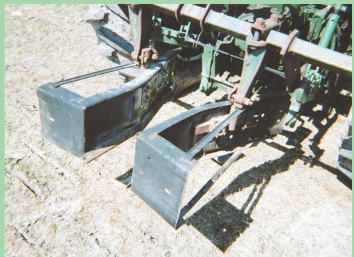
Ron Rosandich bolted a pair of modified car ramps on an old cultivator to make "hillers" for his pumpkin patch. Ramps are spaced about 15 in. apart.
