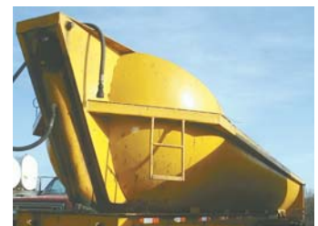
A large hydraulic cylinder raises bed up to a 48-degree angle. Tank's curved shape helps material slide out easily.
