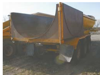
Side swinging gate (left) on back (left) was built out of 2-in. sq. tubing and 1/8-in. thick steel.
