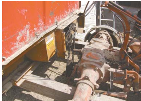
Samuel Yoder uses an Allis Chalmers WD 45 tractor to self propel an old stationary TMR mixer (above). Tractor's pto is used to chain-drive the mixer.
