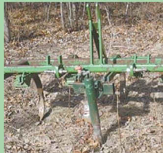
Don Ramberg welds trailer tongue jacks on front of 3-pt. implements such as his cultivator (left) and snowblower.
