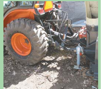
Don Ramberg welds trailer tongue jacks on front of 3-pt. implements such as his cultivator (left) and snowblower.
