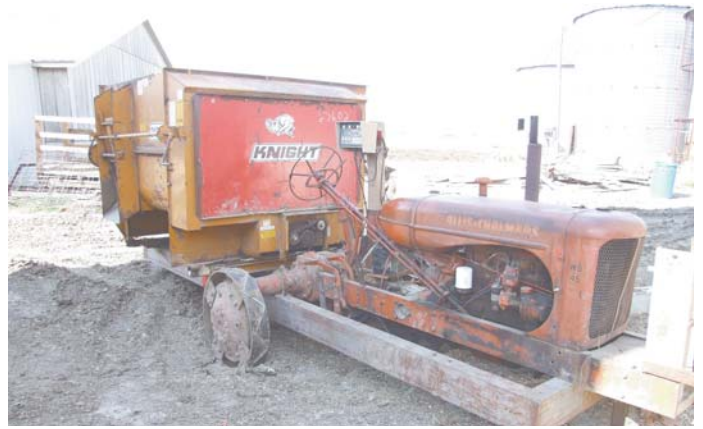
Samuel Yoder uses an Allis Chalmers WD 45 tractor to self propel an old stationary TMR mixer (above). Tractor's pto is used to chain-drive the mixer.
