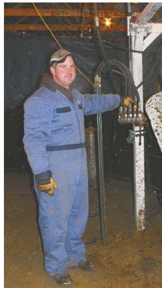
Squeeze chute operator uses valves to open or close hydraulic gates on 4 different pens. Each gate has a 2 by 20-in. hydraulic cylinder mounted at the corner.
